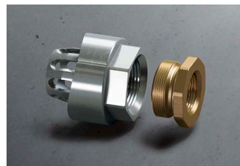
The press-in connection is suitable for steel pipes in accordance with DIN EN 10220/10255 and is available for steel pipe dimensions of 1 1/2", 2", 2 1/2", 3", 4", 5" and 6". It is equipped with a 3/4" internal thread. A reducer for a 1/2" internal thread is also available.
