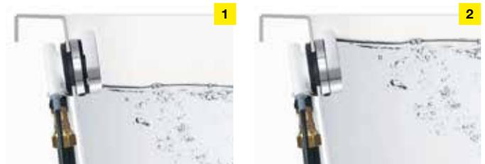
Fig. 1: Without overflow raiser function, the water flows off directly at the bottom of the drain.
